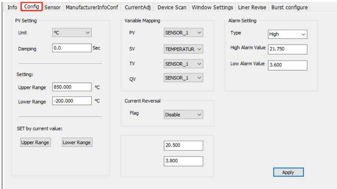
Figure 3.4 Configuration information configuration interface
