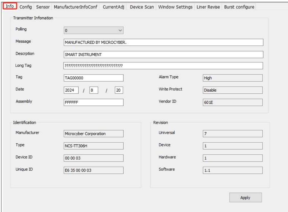
The screenshot shows a software interface with a menu bar at the top containing: Info (highlighted), Config, Sensor, ManufacturerInfoConf, CurrentAdj, Device Scan, Window Settings, Liner Revise, and Burst configure. Below the menu bar, the interface is divided into three main sections:
