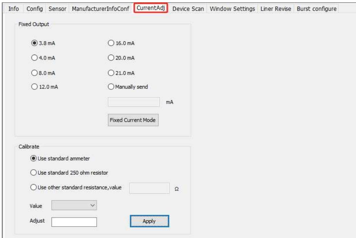
Figure 3.6 Current calibration interface
